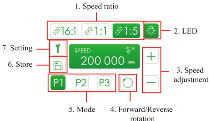
5.6.1 Select speed ratio through touching key “1”. The color of the key will change when touching the key.
