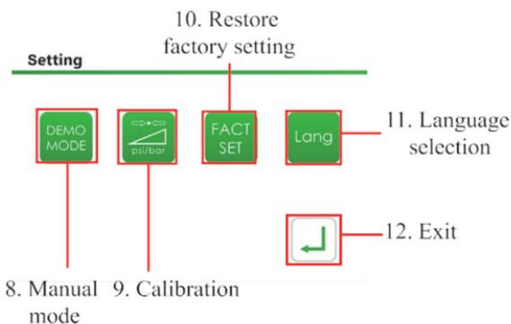
5.7.1 In setting interface, touch key “8” Manual Mode key to enter manual mode interface. Under the manual mode state, the rotation of motor can be directly controlled without foot pedal. Touch Speed Ratio key to select corresponding speed ratio. Touch Speed key to adjust the speed. Touch Start key, Stop key, Forward/Reverse Rotation key, and LED key to control the output of motor. Touch the Exit key to exit the manual mode interface.
