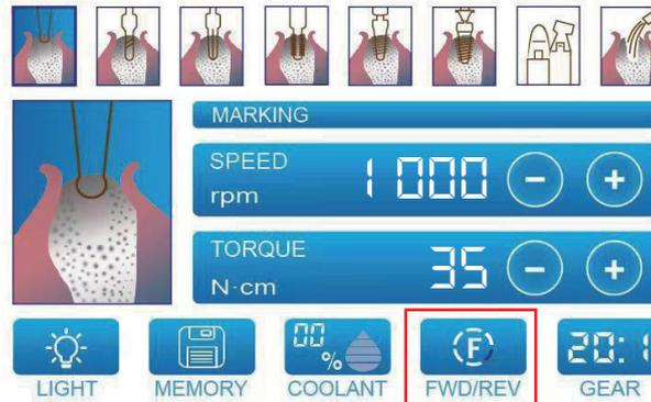
Touch the key shown above to change the rotating direction of motor.
