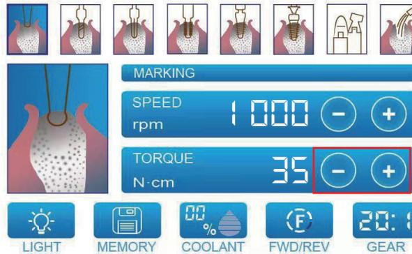
14 Touch the “Torque” (+, -) key to adjust maximum torque output of motor. The torque will change each time after touching the “Torque” key. Long press the “Torque” key to accelerate the change of torque setting value.
