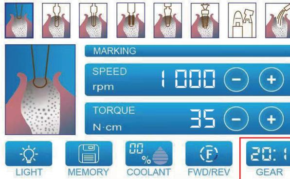
Adjust by pressing the "Speed Ratio" button to match the gear ratio of the handpiece to be used.
