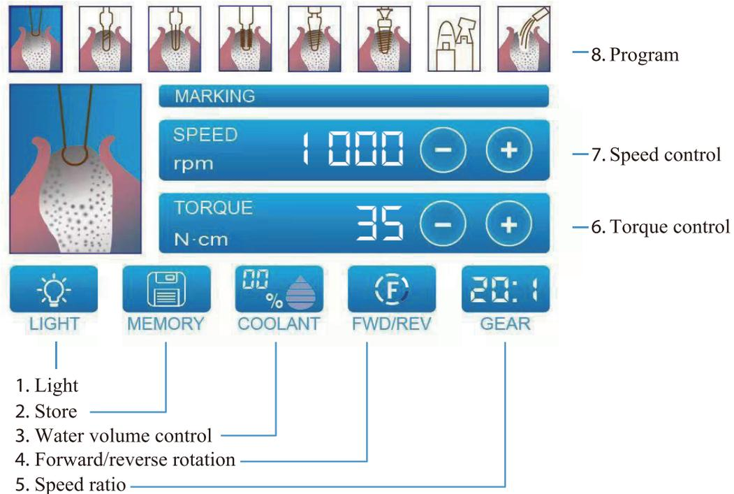
1. Light key      Motor LED switch; circular touch to control the on/off of LED.
