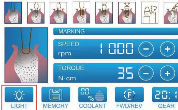
Touch the “LED” button to for setting to determine the on or off state of LED while stepping on foot pedal. The state of LED will change once after each touch. Only the device with LED owns this function.
