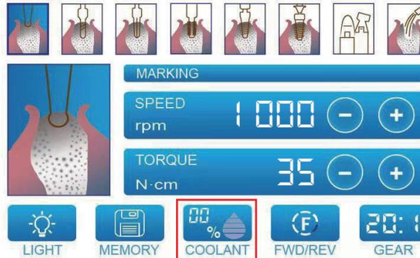
Touch the “Water volume” key on the screen to adjust. There are 6 water levels. The water level will change to the next level after each touch.
