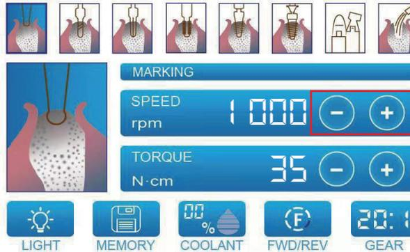
Touch the “Speed” (+, -) key to adjust motor speed. The speed will change each time after touching the “Speed” key. Long press the “Speed” key to accelerate the change of speed setting value.
